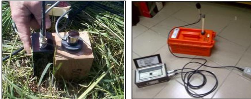
*Figure 3:* Accelerometer installed at site-left (Bahrekazemi, 2004) and seismograph used by the author-right
