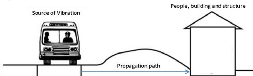
*Figure 1:* Illustration of propagation of ground-borne vibration towards buildings and structures
