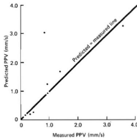
*Figure 5: Predicted and measured vertical PPV at building foundations due to HGVS passing over road surface irregularities (Watts, 1990)*
